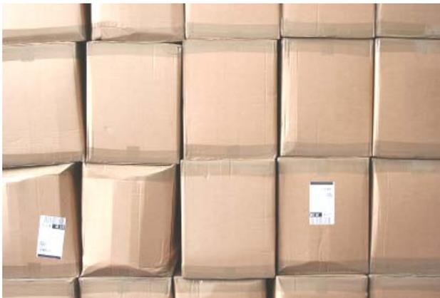
At the top the stack seems fine, but as you look down towards the base of the stack, you will see a badly bruised, damaged carton about to collapse.
